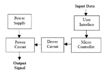
Figure 2.1: Basic Block Diagram of the s/w controlled inverter
