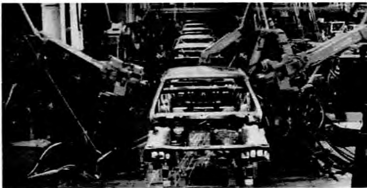
Figure 2.2: Industrial robots spot weld automobile bodies on an assembly line
