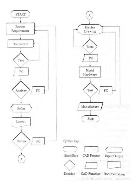
Figure 2.1- Flow Diagram of CAD methodology
