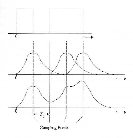
Figure 1.3.6 Examples of ISI on received pulses in a communication system
