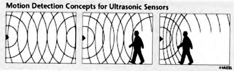
Figure 2-2 A simplified wave patterns in an empty room illustrates the motion detection concepts for ultrasonic sensors.
