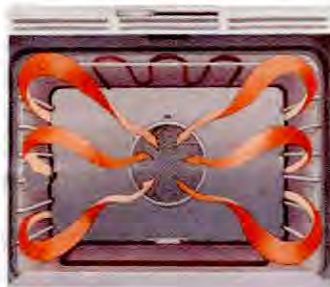
Figure 2.2: Heat flow in the convection oven.
