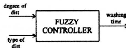
Figure 2.2: Fuzzy controller block diagram
