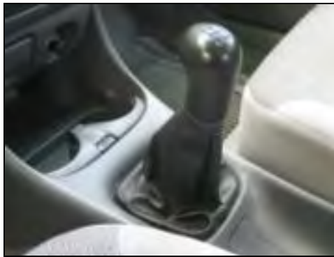
Figure 2.1: Five Speed Shift Stick of a Manual Transmission Car
