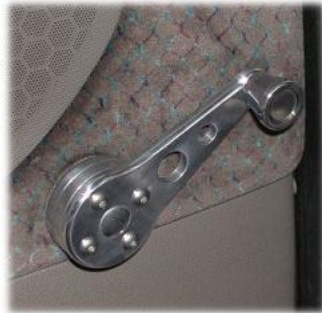
Figure 2.1: Hand-crank car window (Source: http://en.wikipedia.org/wiki/Crank )
