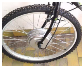
Figure 1.1: 24V generator (previous work)
