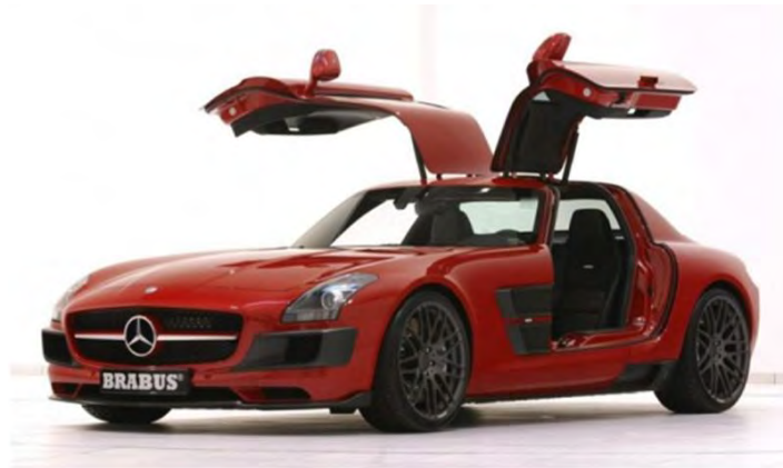
Figure 5: Gull-wing door ( www.carsrevolution.com )
