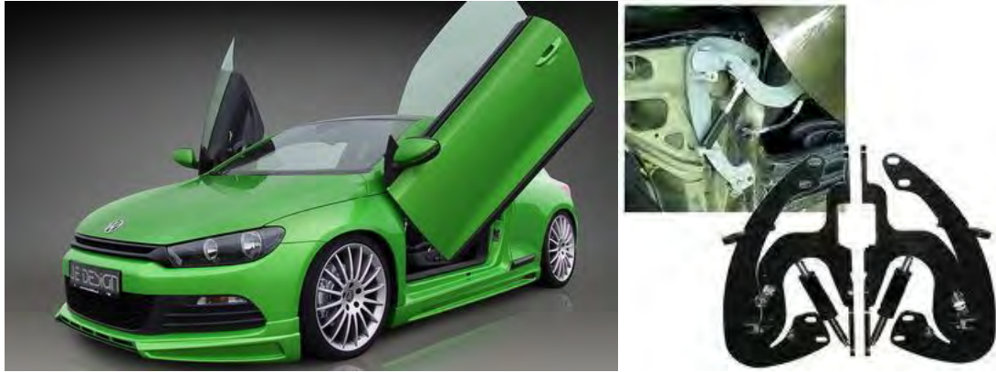
Figure 4: Scissor door hinge ( www.boldride.com )
