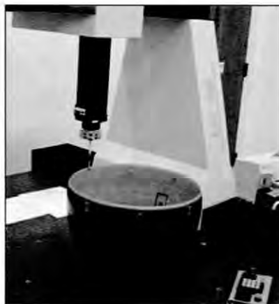
Figure 2. 3: Contact RE Using CMM Machine [5]
