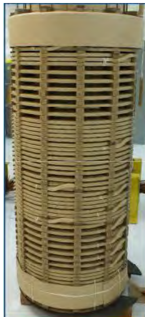
Figure 2.3 Axial displacement of winding [4]
