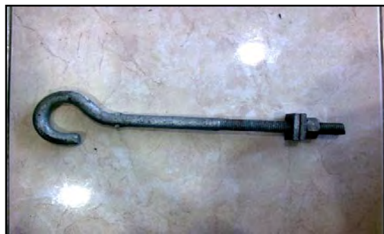
Figure 2.1: ABC Suspension Hook
