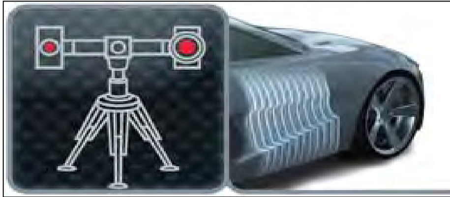
Figure 1.2: This fringe-based white light projection digitizer is combined with optical tracking EFR (Anon, 2010h)
