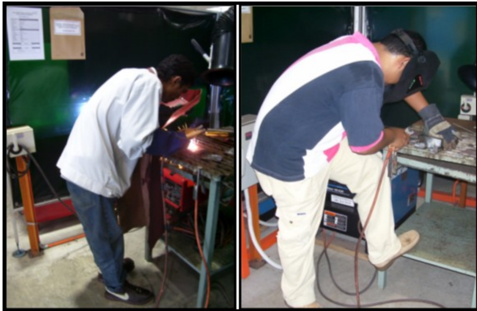
Figure 1.1: Working Posture Adopted by the Students and Staffs in Faculty of Manufacturing Engineering electric arc welding workstation
