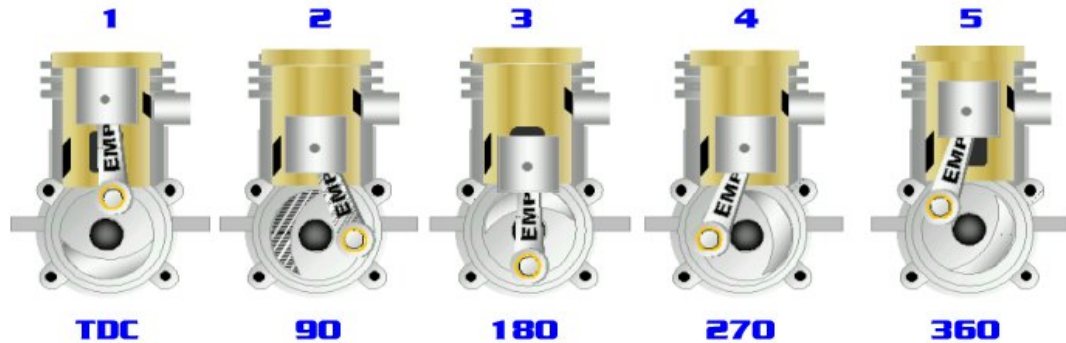
Figure 2.1 Step of Piston Rotation
