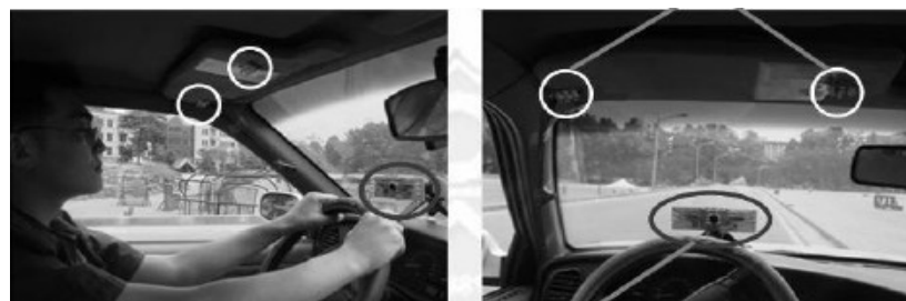
Figure 2.3.1(b): Configuration of the Camera and the Infrared Illuminators [1]
