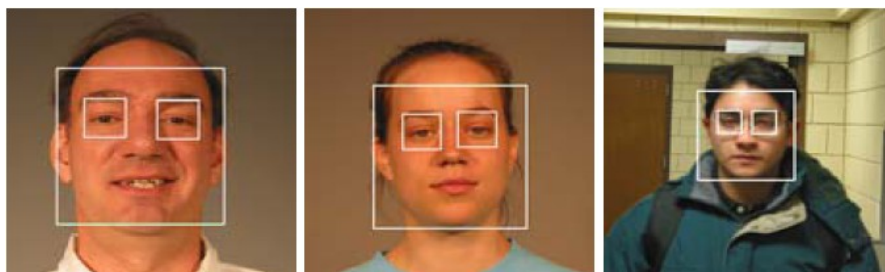
Figure 2.2.2(a): Face and Eye Detection Results
