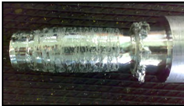
Figure 4.5: Coarse and uneven surface
