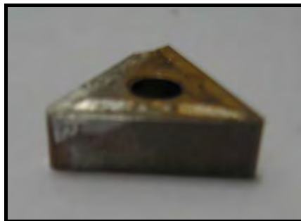
Figure 4.6: Condition of cutting tool after DOE for turning process
