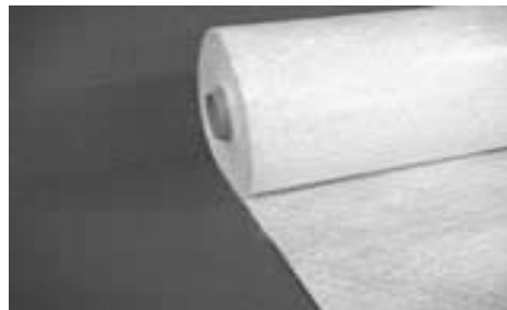
Figure 2: Chopped strand mat (CSM)
