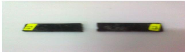
**Figure 4.9(b)** Charpy failure mode with 2% of nano  $\text{CaCO}_3$
