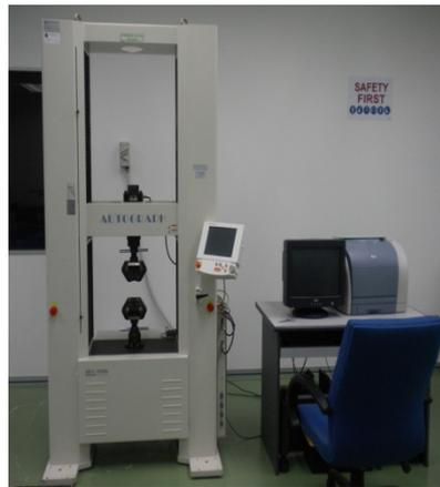
**Figure 3.5 :** Shimadzu Universal Tensile Machine AG-1
