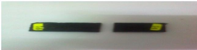
**Figure 4.9(c)** Charpy failure mode with 4 % of nano  $\text{CaCO}_3$
