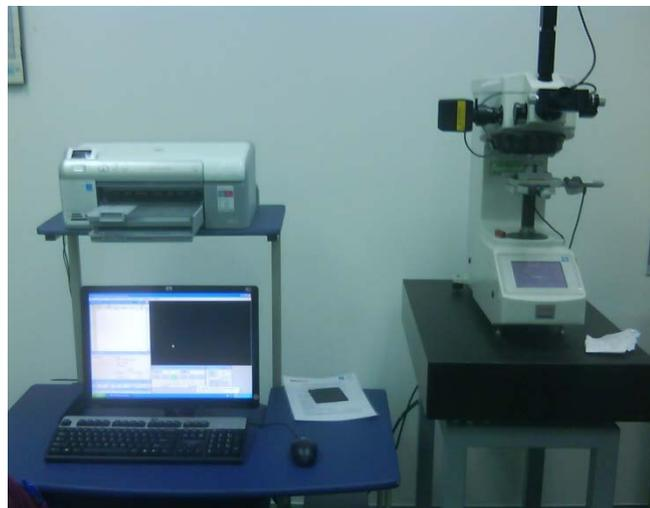
**Figure 3.9:** Vickers micro hardness Test (UTeM)
