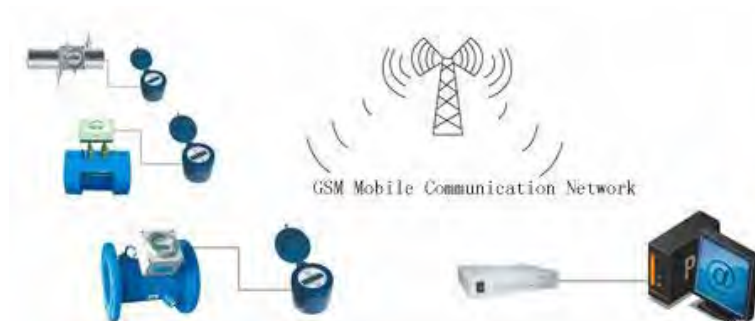
Figure 1.1 Example of wireless water meter system from digital meter to control station.
