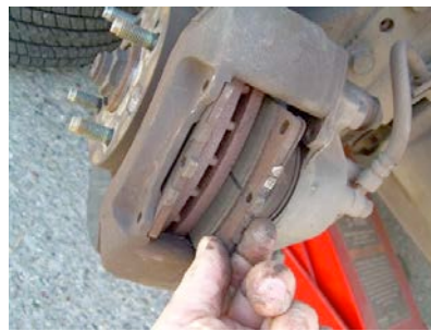
Figure 2: Faulty of the brake pads (“Disc Brake Drag” www.dnr.louisiana.gov )
