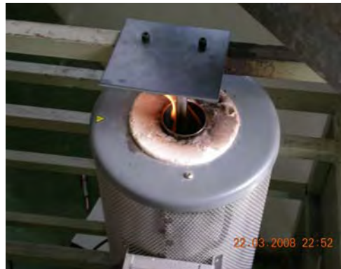
Figure 5.1 Flaming occurred at temperature 500°C by using the compression method
