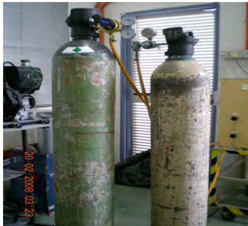
Figure 3.18 Nitrogen and carbon dioxide gas tank
