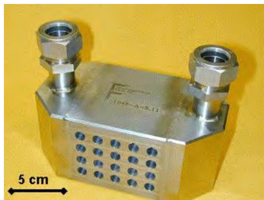
Figure 1.3 Electrically powered microstructure heat exchanger used in the production of bio-diesel (Source: Brandner, J. J. et. al. 2006)
