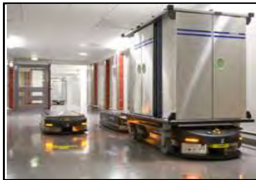
Figure 2.1: TransCar AGV (Swisslog.com).
