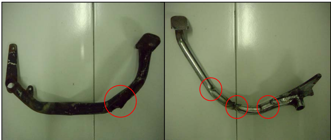
Figure 1.2: Failure at motorcycle brake pedal
