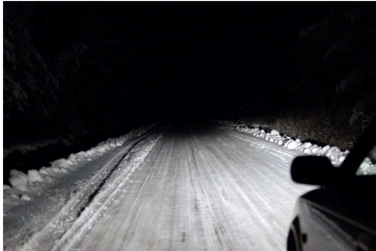
Figure 2.1 E-code dipped/low beam.
