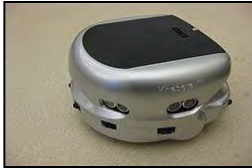
Figure 2.1: Khepera mobile robot ( robotics.youngester.com/2009/10/...ots.html )
