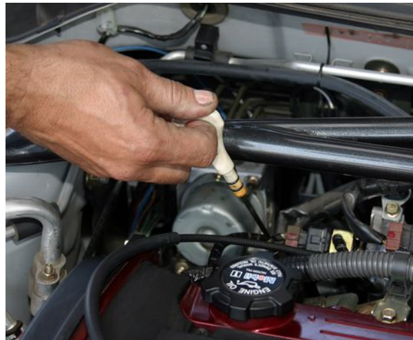
Figure 9: Oil Level Is Checked Using Dipstick [5]
