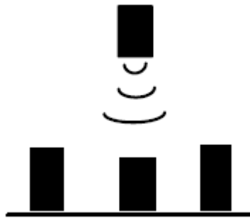
Figure 2.4.3 Application of ultrasonic in height difference
