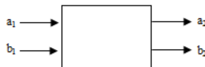
Figure 2.5: Two port network
