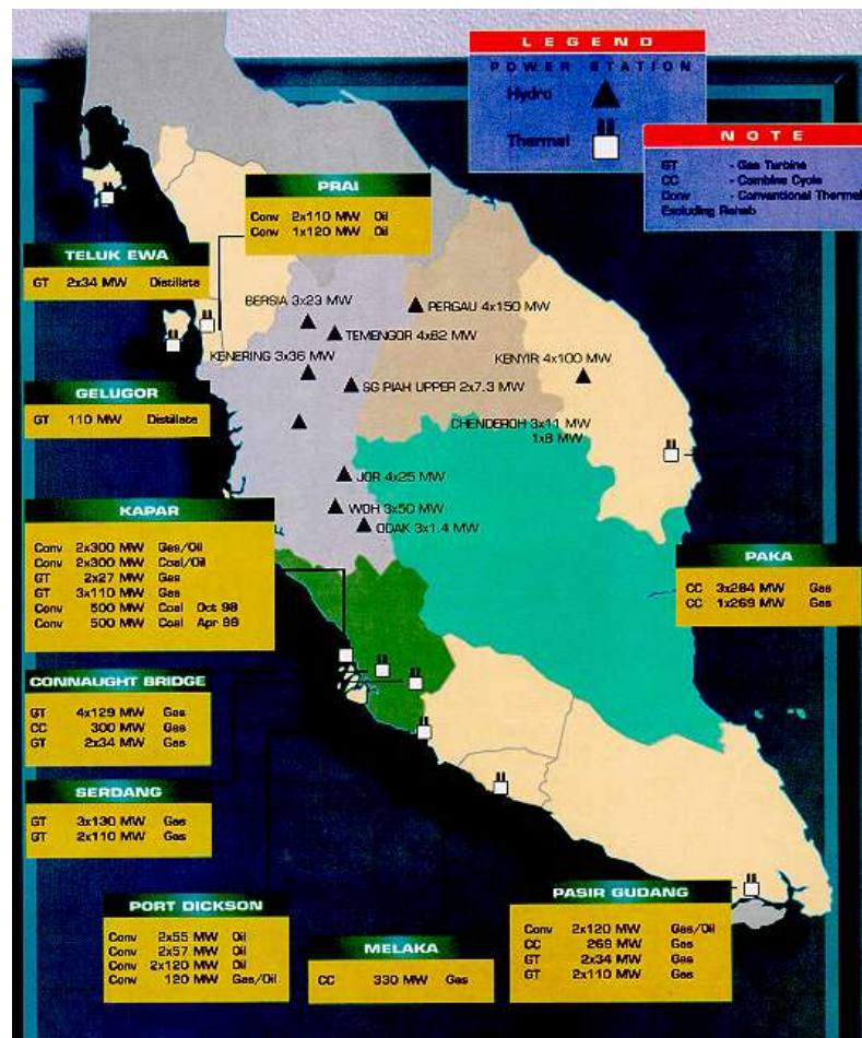
FIGURE 2.0: The power plants (thermal, gas and hydro) in Peninsular Malaysia (Source: TNB Kenyir)
