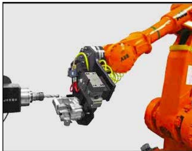
Figure 2.2: Water pump deburring cell setup (George, Z. et. al: (2008).
