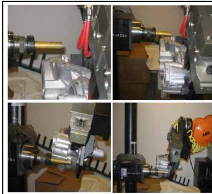
Figure 2.3: Pictures taken while the tool is in force control mode and programmed to follow the edge of the water pump (George, Z. et. al: (2008).
