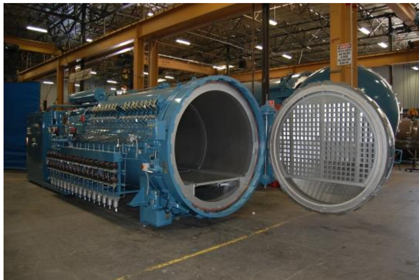
Figure 1. Industrial Horizontal Autoclave (Source : ASC Process Systems,2006)
