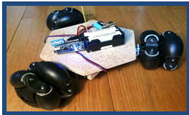
Figure 2- 1: Tricycle Robot Using Omni-Wheels
