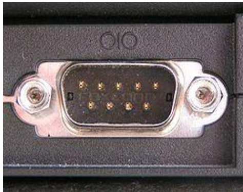
Figure 1 : A male DE-9 connector used for a serial port on a IBM PC compatible computer
