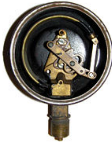
Figure 2.3 Bourdon meter (with back cover removed)
