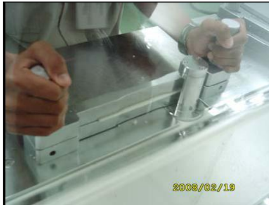
Figure 3.15: Cutting Process of Tensile Specimen
