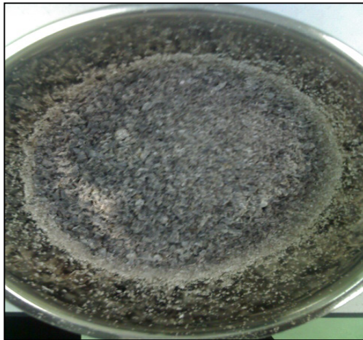
Figure 3.12: Blend Material after crushing (particle form)
