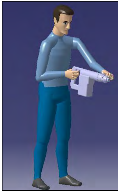
Figure 25: First posture using existing breaker
