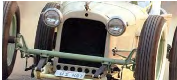
Figure 2.1: Front leaf spring loaded on vintage hotrod vehicle
