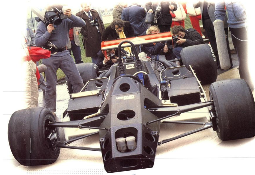
Figure 1: The original composite F1 chassis, McLaren MP4-1 (Savage, 2008)
