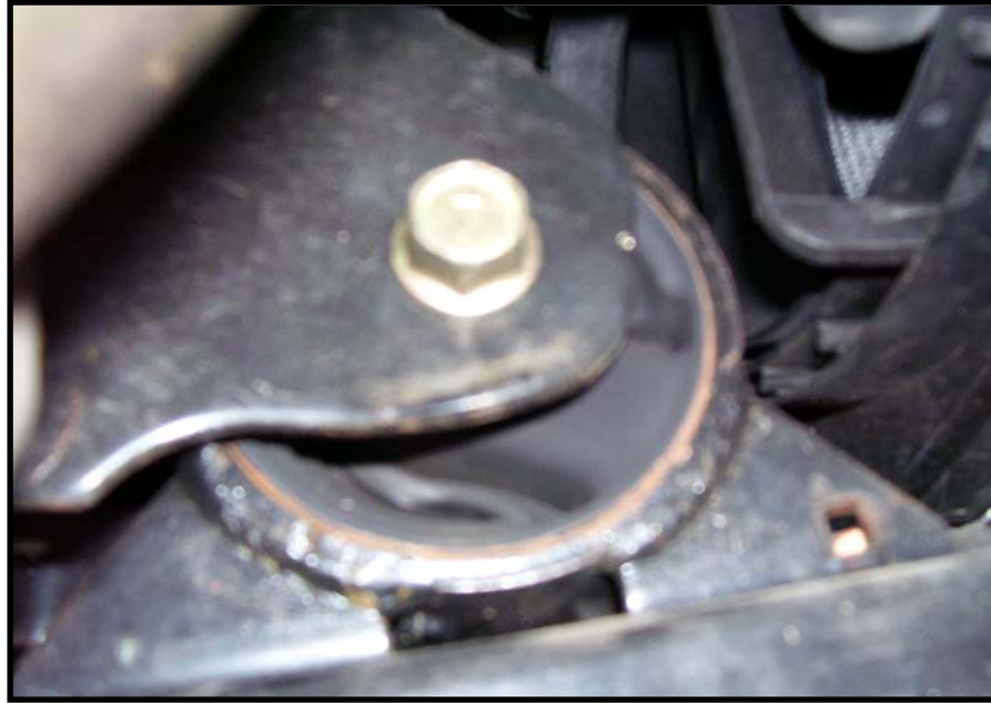
Picture 3. Engine mounting, located at the bottom of engine
