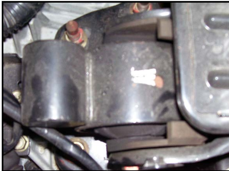
Picture 2. Engine mounting at the right side, on the top of gearbox
