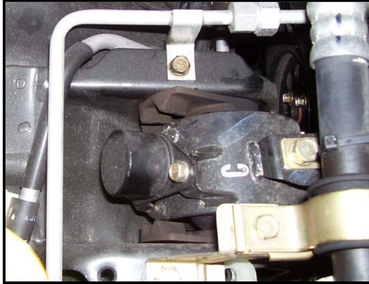
Picture 1. Engine mounting at the left side of engine block
