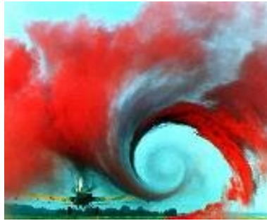
Figure 2.1: A vortex is created by the passage of an aircraft wing.
