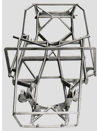
Figure 2.2: The tubular chassis of the 3500 GT (Source: www.maserati-alfieri.co.uk )
