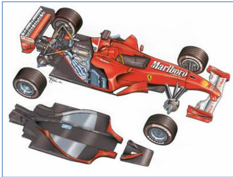
Figure 1 : Composite chassis for Formula 1 race car (Source: http://www.one-pablo.com/technique/chassis1.jpg )
