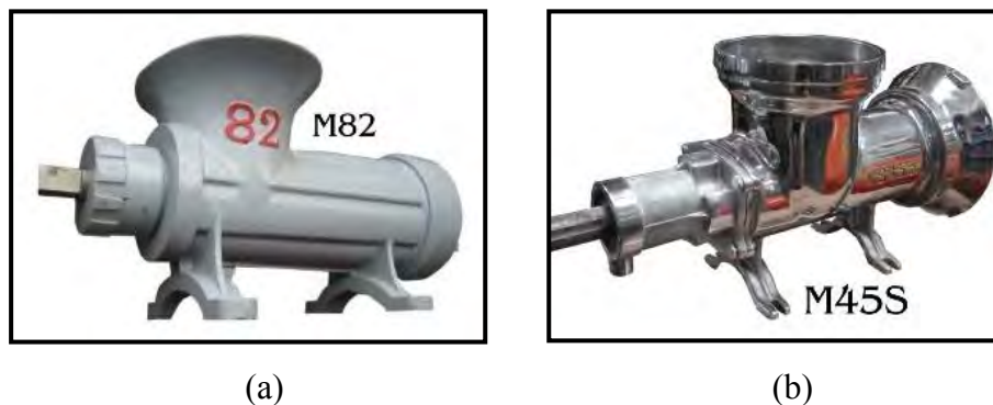
Figure 2.1: (a) Meat Mincer Size M82, (b) Meat Mincer Size M45S (Stainless Steel)
