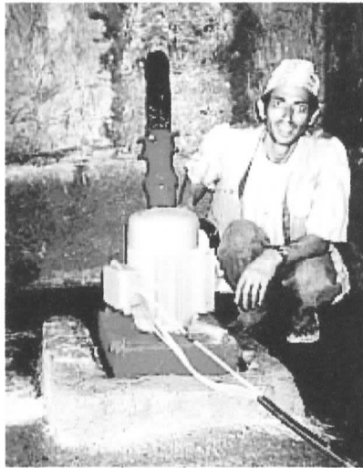
Figure 2.1: The 'Peltric Set' has provided many rural village with an economical electricity supply in Nepal
