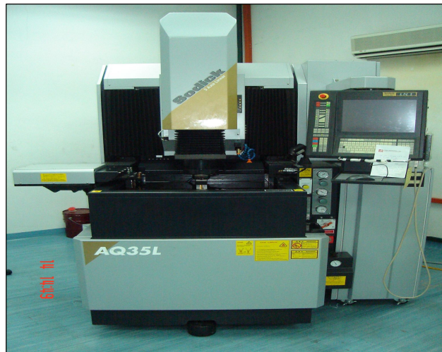
Figure 1.1: Die-Sinking EDM (MODEL: AQ35L SODICK)
