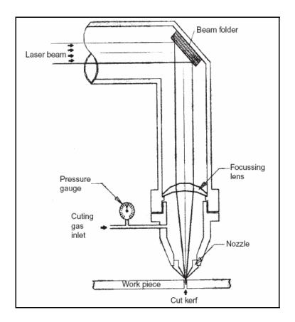
Figure 2.6: Basic Diagram of Laser Cutting Operation [7]
