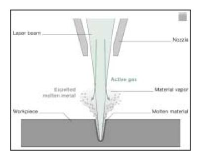
Figure 2.5: The laser drilling operation; the laser melts and vaporizes the material. The vapour pressure expels the molten material out from the hole.
