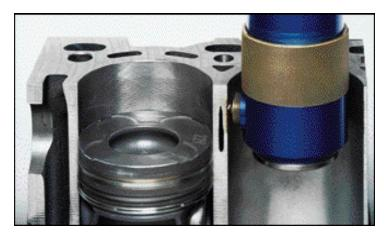
Figure 1.2: Laser texturing of engine cylinder walls [3].
