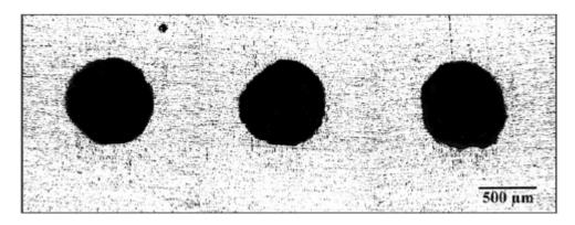
Figure 1.1: Variation of entrance geometry of laser percussion drilled holes under the same operating parameter setting [2].
