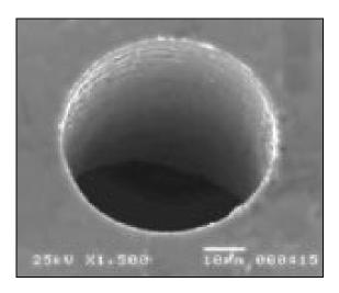
Figure 2.7: 150 micron diameter hole in silicon [16]
